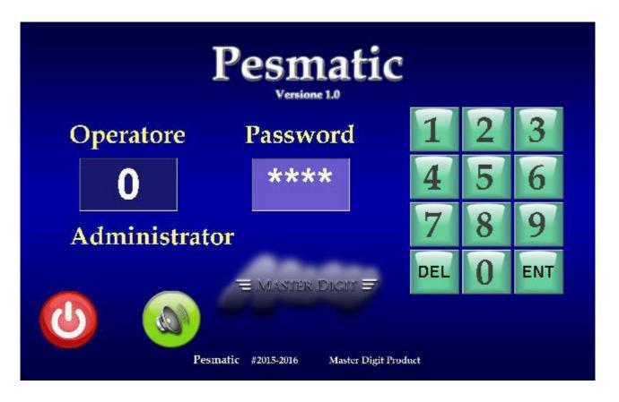
With the red button on the bottom left of the screen you can switch off the Pesmatic automatic balance as seen above, while the green button next to the screen will enable or disable the audio guide of the Pesmatic automatic balance.
