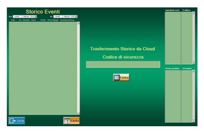
In the window below the **Security Code** you enter the PC keypad, the previously obtained code (page 14) from the Pesmatic automatic balance (*after saving the balance statistic on the dedicated Cloud*
