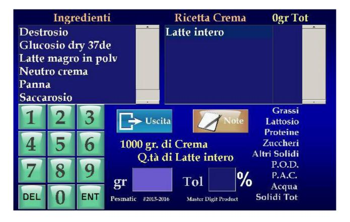
To insert a new recipe, select the first ingredient in the upper-left window of the screen where all the ingredients included in the Pesmatic automatic balance are displayed. The ingredient will be returned to the window at the top right of the screen and the **Note** button will appear, pressing which you can, by means of a submenu, enter a comment on the preparation of the ingredient for this recipe with a 250-character text.
