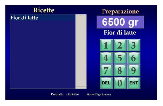
Using the numeric keypad at the bottom right of the screen, enter the amount to be prepared in grams by displaying the weight entered in the upper-right window of the screen, press the **ENT** key to confirm the insertion.
