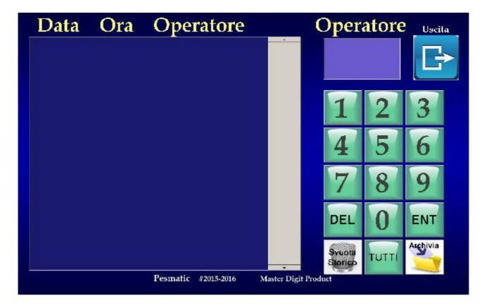
Using the numeric keypad on the right side of the screen, enter the number of the operator who needs to know the time accesses on the Pesmatic automatic balance. Pressing **ENT** (Enter) after entering the operator number will appear in the list on the left all data for the date, time, operator number, name or code in history from the first access to the last selected operator.
